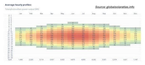
In summary, in 1 day during the month of June, in Chicago, IL, you could harvest 16.58kWh\* of solar energy. Assuming average performance ratio\*, efficiency\*, cloud cover, and weather conditions.
